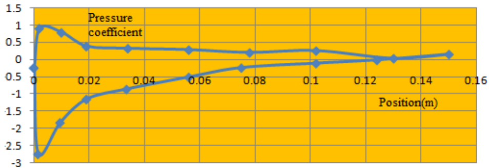
Fig. 2 – The pressure coefficient determined by experiment.
